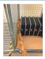
The recycled paper should be placed in the peripheral areas in order to protect the devices during transportation.
