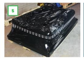
Isolate the pallet with black protective cover. Attach the KO-number and UN 3481 on all sides.
