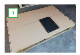
Define the center of the carton by drawing two lines, one crossing the other and place the laptops so they align with the back towards center line facing the side of the pallet.
