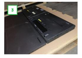
In the next layer place the laptops with screens down. In the third layer the laptops should be placed bottom-to-bottom.
